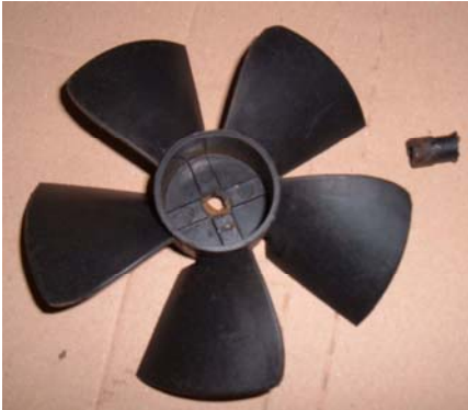
Typically damaged fan blades
